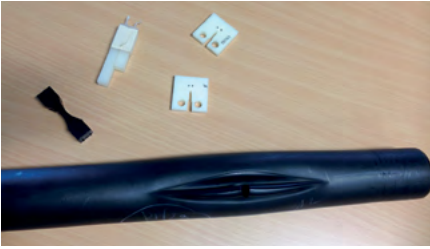
Fig. 1 – A burst pipe with some other tested samples
